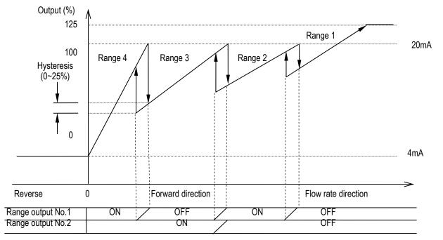
14. Automatic selection of unidirectional flow multi-range with an internal signal
